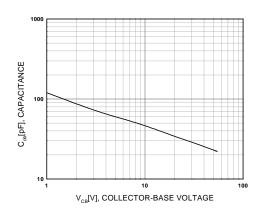
Figure 4. Collector Output Capacitance
