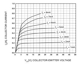
Figure 1. Static Characteristic
