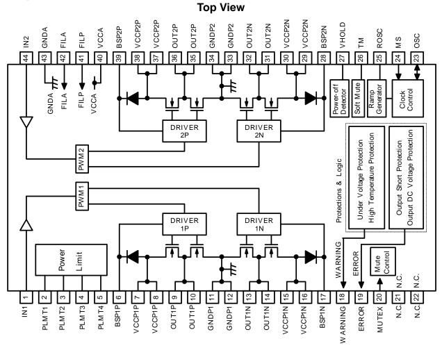
Fig. 23 Pin Assignment Diagram
