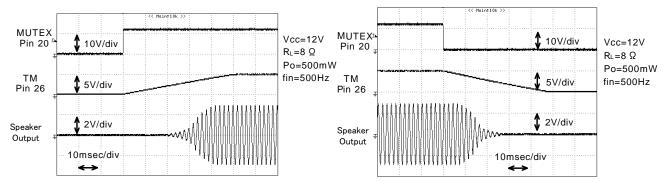
Fig. 13 Wave form when Releasing Soft-mute
