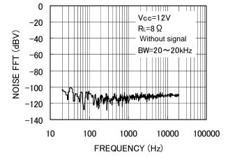
Fig. 12 FFT of Output Noise Voltage
