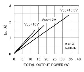
Fig. 10 Current consumption - Output power
