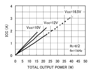
Fig. 22 Current consumption - Output power
