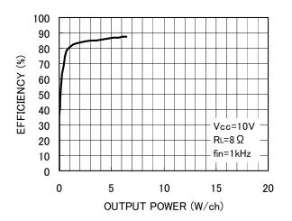
Fig. 7 Efficiency - Output power
