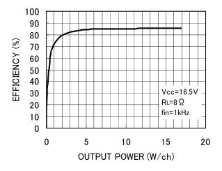
Fig. 9 Efficiency - Output power
