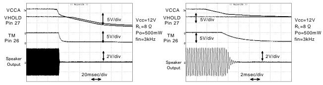
Fig. 15 Wave form on Instantaneous Power Interruption (20msec / div)
