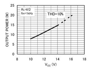
Fig. 18 Output power - Power supply voltage
