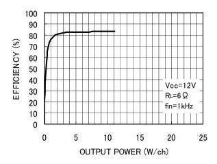
Fig. 20 Efficiency - Output power
