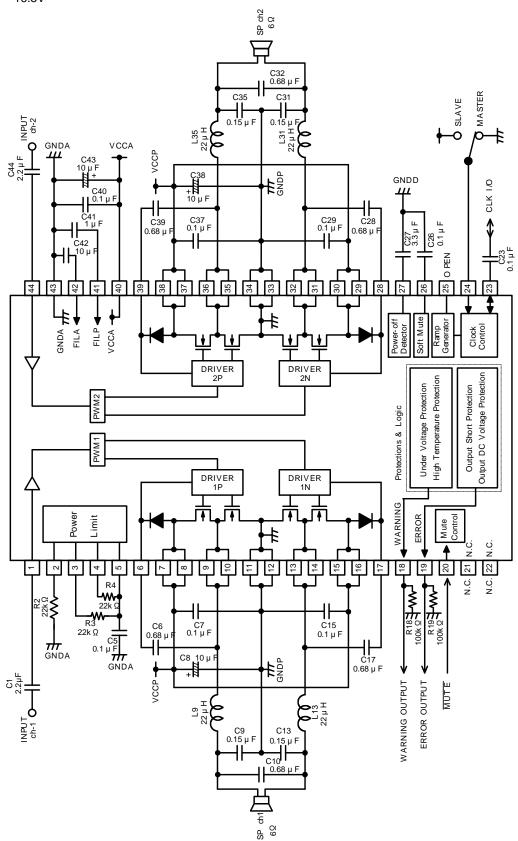
Fig. 25 Circuit Diagram of Stereo Operation with  $6\Omega$  Load
