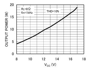
Fig. 6 Output power - Power supply voltage
