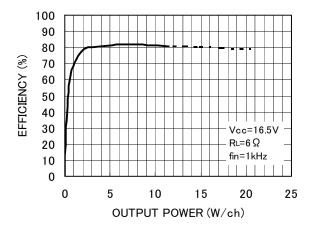
Fig. 21 Efficiency - Output power
