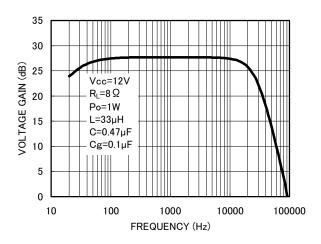
Fig. 3 Voltage gain - Frequency
