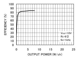
Fig. 19 Efficiency - Output power
