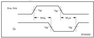
Waveform 1. Propagation delay for inverting outputs
