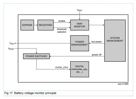
The value of the critical level can be configured to 2.3 V or 2.75 V by an EEPROM setting. This value has a typical hysteresis around 150 mV.
