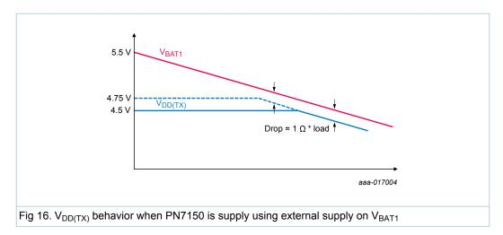
Figure 16 shows the behavior of  $V_{DD(TX)}$  depending on  $V_{BAT1}$  value.
