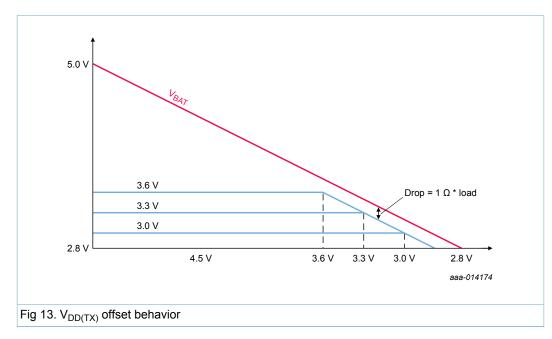
Figure 13 shows  $V_{DD(TX)}$  offset disabled behavior for both cases of  $V_{DD(TX)}$  programmed for 3.0 V, 3.3 V or 3.6 V.
