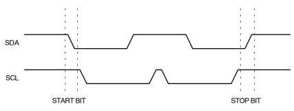
Figure 4. Start/Stop Timing
