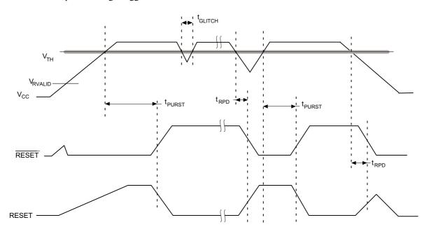
Figure 1. RESET Output Timing
