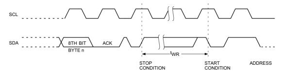
Figure 3. Write Cycle Timing
