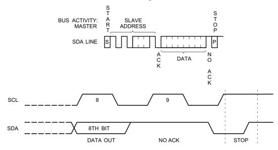
Figure 9. Immediate Address Read Timing
