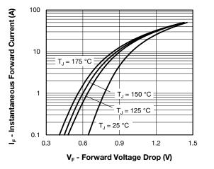
Fig. 1 - Typical Forward Voltage Drop Characteristics
