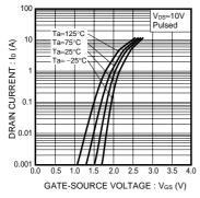
Fig.4 Typical Transfer Characteristics
