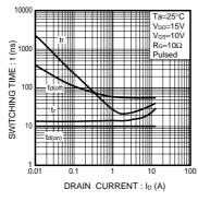
Fig.2 Switching Characteristics
