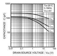
Fig.1 Typical Capacitance vs. Drain-Source Voltage
