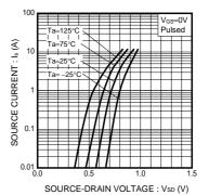
Fig.6 Source Current vs. Source-Drain Voltage
