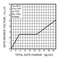
Fig.3 Dynamic Input Characteristics
