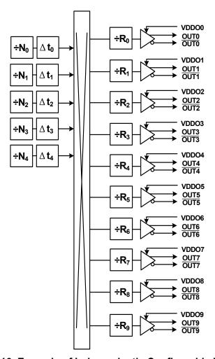
Figure 16. Example of Independently Configurable Path Delays
