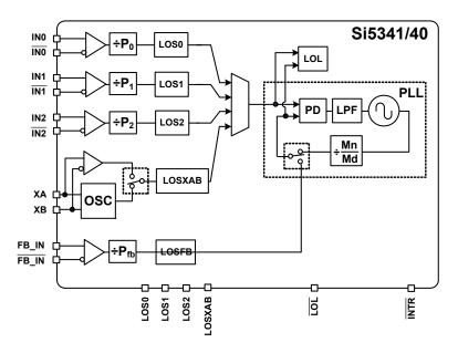
Figure 13. LOS and LOL Fault Monitors
