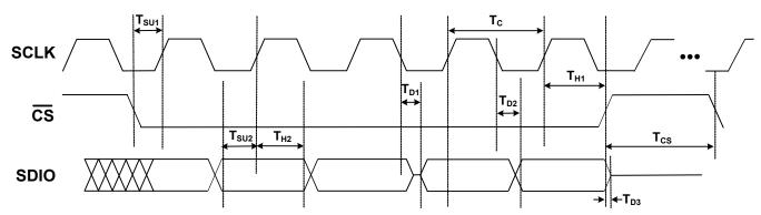
Figure 4. 3-Wire SPI Serial Interface Timing
