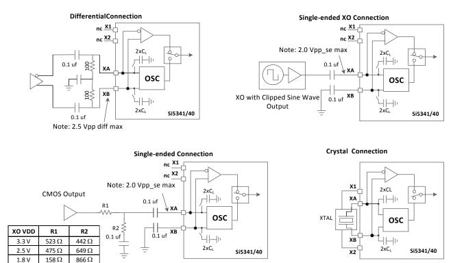
Figure 11. XAXB External Crystal and Clock Connections
