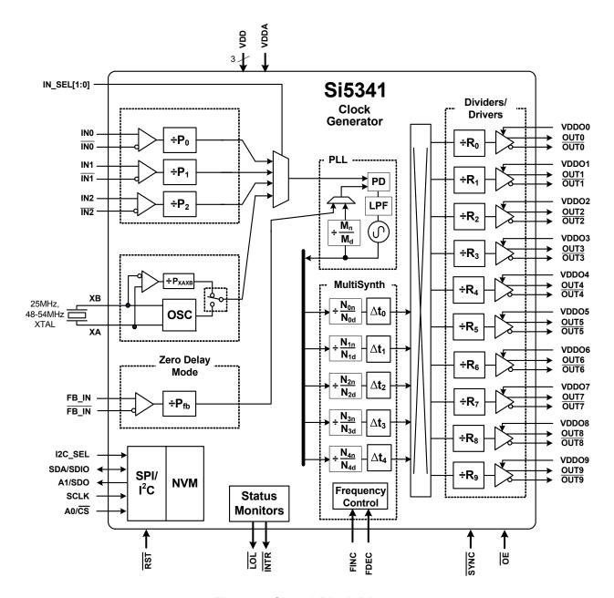
Figure 8. Si5341 Block Diagram
