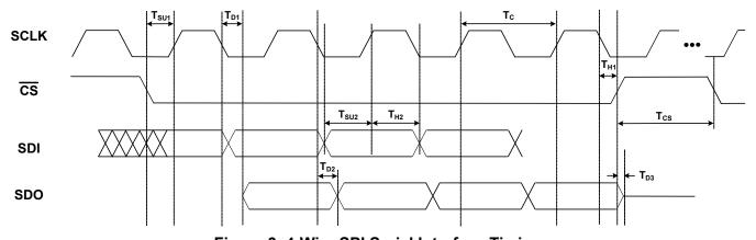
Figure 3. 4-Wire SPI Serial Interface Timing
