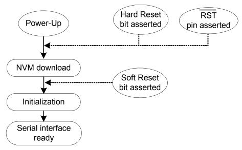
Figure 10. Si5341 Power-up and Initialization
