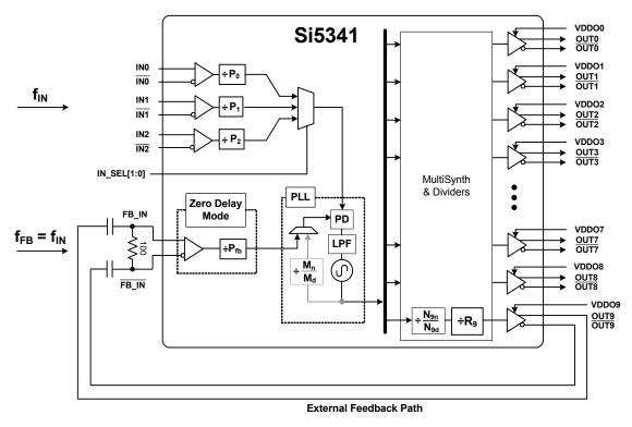
Figure 17. Si5341 Zero Delay Mode Setup
