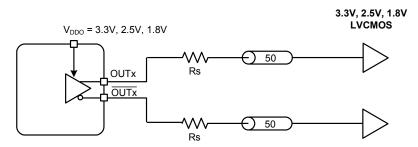
Figure 15. LVCMOS Output Terminations
