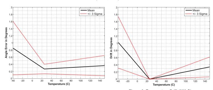
Figure 8: Angle Error Over Temperature (300 G)
