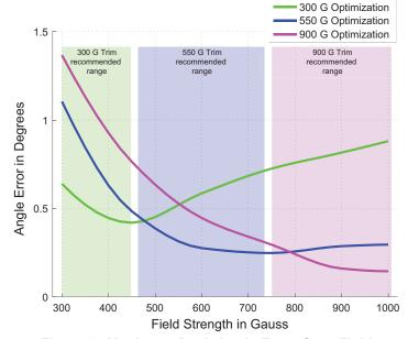
Figure 3: Maximum Peak Angle Error Over Field
