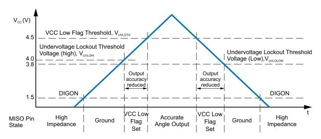
Figure 1: Relationship of VCC and MISO Output
