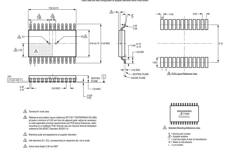
Figure 19: Package LE, 24-Pin TSSOP (Dual Die Version)
