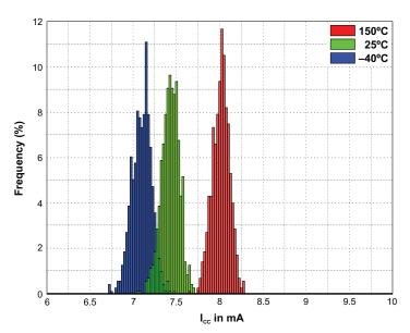
Figure 14:  $I_{CC}$  Distribution Over Temperature  $(V_{CC} = 14.5 \text{ V})$
