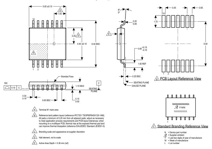
Figure 18: Package LE, 14-Pin TSSOP (Single Die Version)
