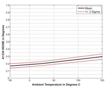
Figure 11: Noise Performance Over Temperature  $(1\sigma, 300 \text{ G})$
