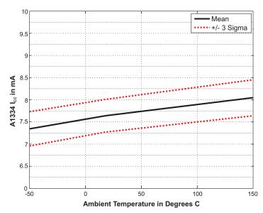
Figure 13:  $I_{CC}$  Over Temperature  $(V_{CC} = 4.5 \text{ V})$
