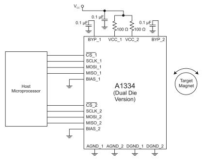
Figure 16: Typical Application Diagram (dual die version) with EMC Suppression Resistor, R<sub>SPLY</sub>, on Supply Line
