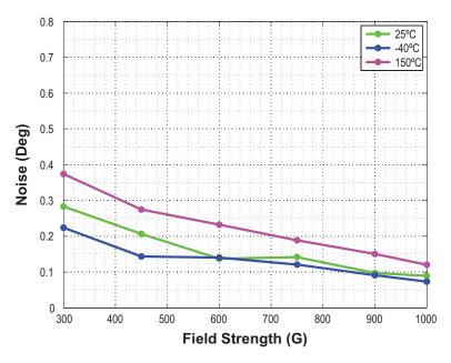
Figure 4: One Sigma Noise over Field Strength
