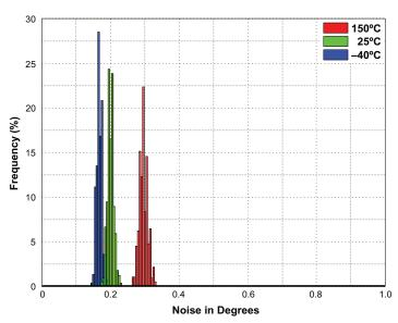
Figure 10: Noise Distribution Over Temperature  $(1\sigma, 300 \text{ G})$
