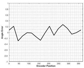
Figure 7: Typical Angle Error versus Absolute Position (300 G, 25°C)
