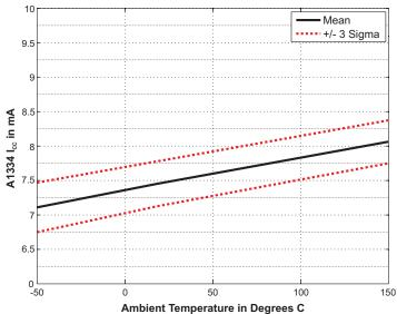
Figure 15:  $I_{CC}$  Over Temperature  $(V_{CC} = 14.5 \text{ V})$
