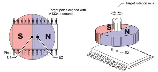
Figure 2: Orientation of Magnet Relative to Primary Die and Secondary Die (dual die version used as example)
