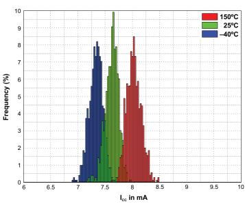
Figure 12:  $I_{CC}$  Distribution Over Temperature  $(V_{CC} = 4.5 \text{ V})$
