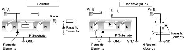
Figure 10. Example of Monolithic IC Structure
