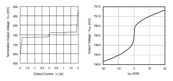
Figure 1. Termination Output Voltage vs Output Current (DDR3)
