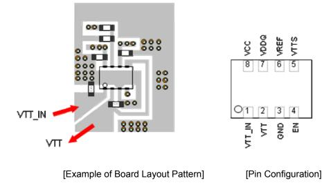
The input capacitor Cin of VTT\_IN should be placed as close as possible to VTT\_IN pin. Similarly, the VTT output capacitor should be placed as close as possible to the IC's pin. As for wiring pattern, make the pin wiring and the GND pattern as wide as possible. As for the metal trace connecting to the inner GND plane, please place many through holes.
