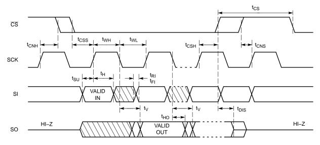
Figure 2. Synchronous Data Timing
