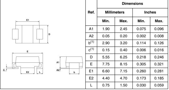
1. Dimensions b and c apply to plated leads
