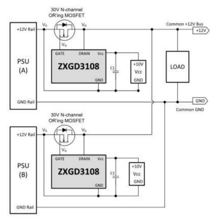
Example of the ZXGD3108 OR'ing Controller in a Redundant High-Side +12V Power Supply Rail with V<sub>CC</sub> Supply
