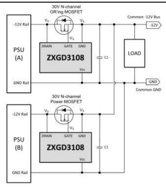
Focus Application of the ZXGD3108 OR'ing Controller is for Redundant Low-Side -12V Power Supply Rail
