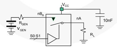
Figure 16. Total Harmonic Distortion
