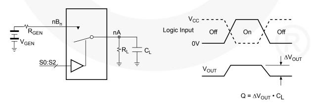
Figure 10. Charge Injection Test
