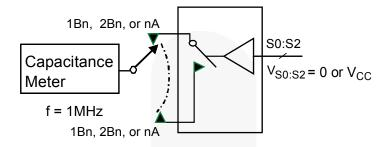
Figure 14. Channel Off Capacitance
