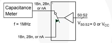
Figure 15. Channel On Capacitance
