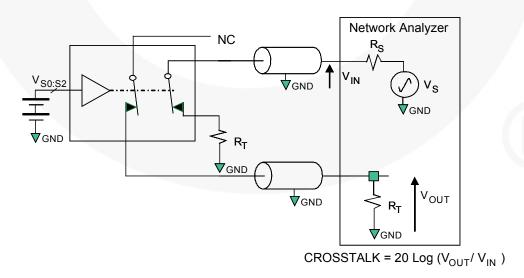
Figure 13. Non-Adjacent Channel-to-Channel Crosstalk
