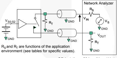
Off-Isolation = 20 Log  $(V_{OUT} / V_{IN})$
