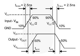
Figure 9. Switch Propagation Delay Waveforms
