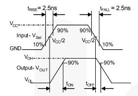
Figure 8. Turn-On / Turn-Off Waveforms
