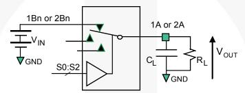
$\rm R_L$  and  $\rm C_L$  are functions of the application environment (see tables for specific values).  $\rm C_L$  includes test fixture and stray capacitance.
