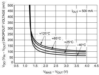
Figure 6. V<sub>IN</sub> Dropout Voltage vs. (V<sub>BIAS</sub> – V<sub>OUT</sub>) and Temperature T<sub>J</sub>
