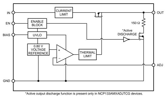
Figure 3. Simplified Schematic Block Diagram - Adjustable Version
