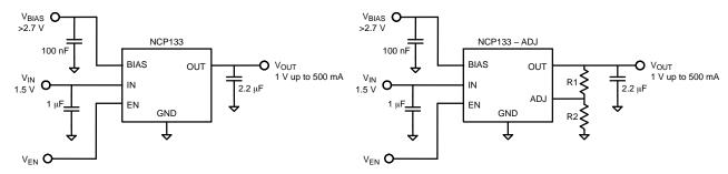
Figure 1. Typical Application Schematics
