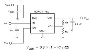
Figure 13. Typical Application Schematics
