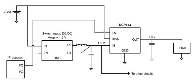
Figure 12. Typical Application: Low-Voltage DC/DC Post-Regulator with ON/OFF Functionality
