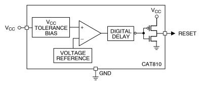
Figure 1. Block Diagrams
