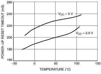
Figure 2. Power-up Reset Timeout vs. Temperature
