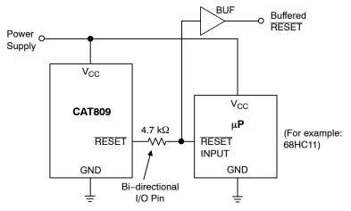
Figure 10. Bi-directional Reset Pin Interfacing
