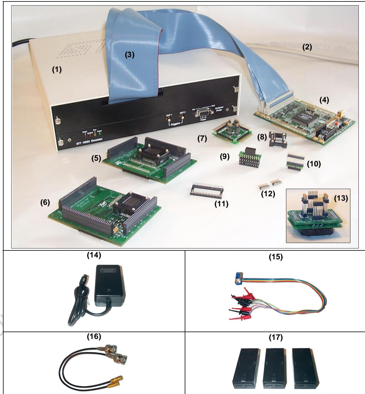
Figure 2: Main components of ST7MDTU2-EMU2B emulator kit
