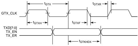
Figure 10. GMII Transmit AC Timing Diagram
