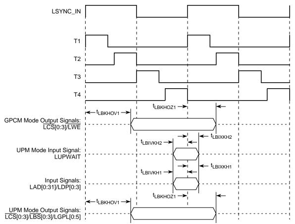
Figure 28. Local Bus Signals, GPCM/UPM Signals for LCRR[CLKDIV] = 4 (DLL Enabled)
