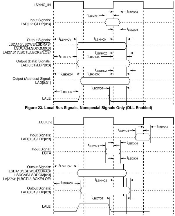
Figure 24. Local Bus Signals, Nonspecial Signals Only (DLL Bypass Mode)
