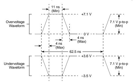
Figure 4. Maximum AC Waveforms on PCI interface for 3.3-V Signaling
