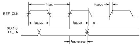
Figure 15. RMII Transmit AC Timing Diagram
