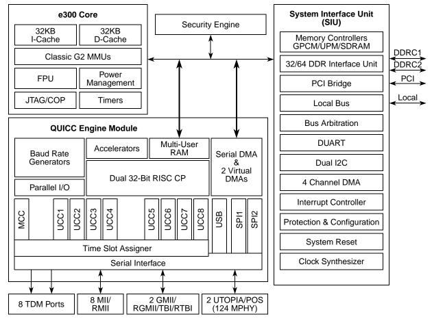
Figure 1. MPC8360E Block Diagram
