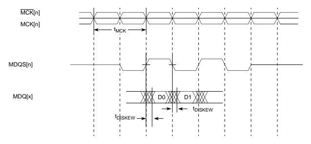
Figure 6. DDR Input Timing Diagram
