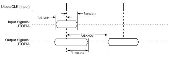
Figure 47. UTOPIA AC Timing (External Clock) Diagram
