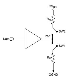
Figure 57. Driver Impedance Measurement
