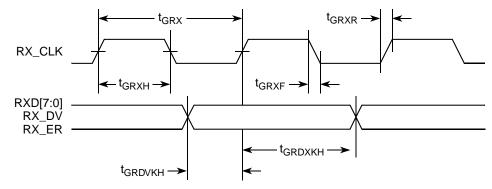
Figure 11. GMII Receive AC Timing Diagram
