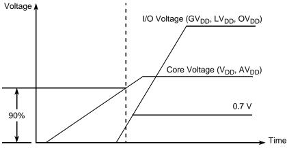
Figure 5. Power Sequencing Example
