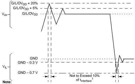
1. Note that  $t_{\mbox{interface}}$  refers to the clock period associated with the bus clock interface.
