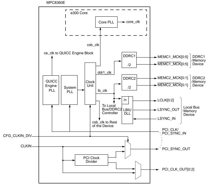
Figure 54. MPC8360E Clock Subsystem
