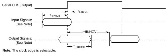
Figure 51. AC Timing (Internal Clock) Diagram
