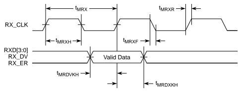
Figure 14. MII Receive AC Timing Diagram
