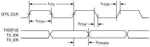
Figure 18. TBI Transmit AC Timing Diagram
