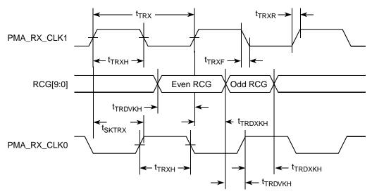
Figure 19. TBI Receive AC Timing Diagram
