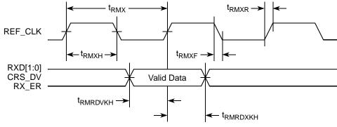
Figure 17. RMII Receive AC Timing Diagram
