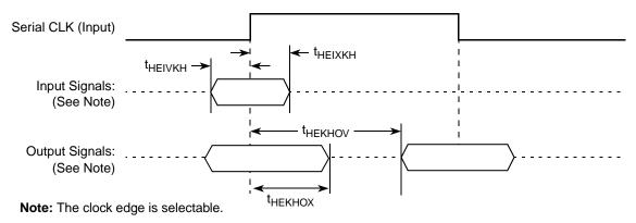
Figure 50. AC Timing (External Clock) Diagram
