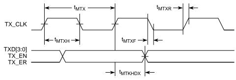
Figure 12. MII Transmit AC Timing Diagram
