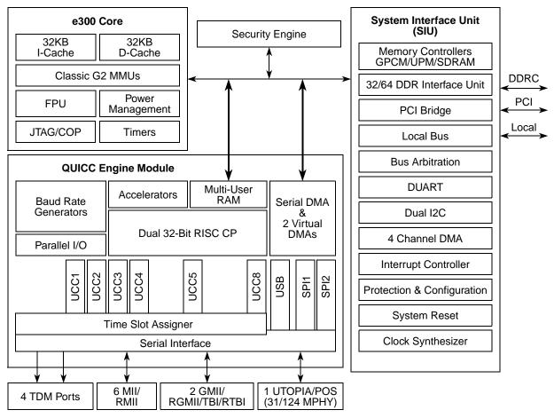
Figure 2. MPC8358E Block Diagram
