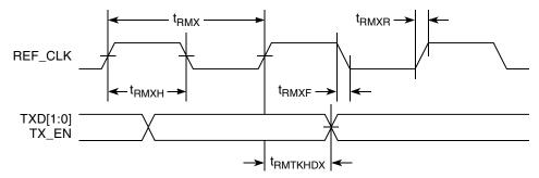
Figure 15. RMII transmit AC timing diagram
