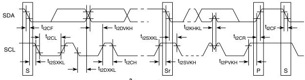
Figure 31. I<sup>2</sup>C bus AC timing diagram
