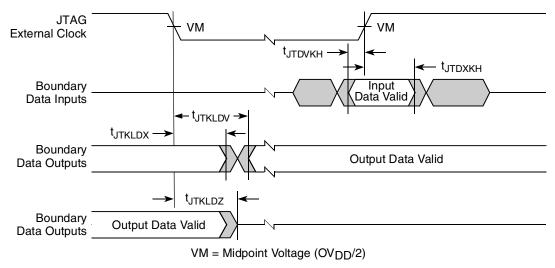
Figure 40. Boundary-Scan timing diagram
