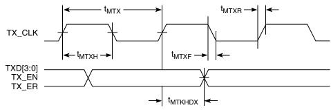
Figure 12. MII transmit AC timing diagram
