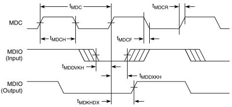
Figure 17. MII management interface timing diagram
