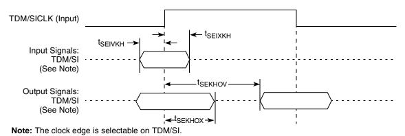
Figure 19. TDM/SI AC timing (external clock) diagram
