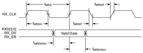
Figure 13. MII receive AC timing diagram
