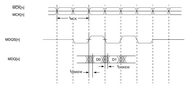
Figure 4. DDR input timing diagram
