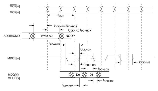
Figure 6. DDR2 SDRAM output timing diagram
