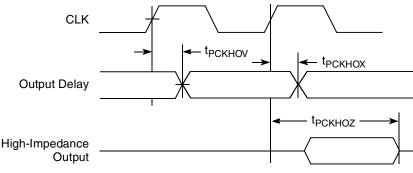
Figure 25. PCI output AC timing measurement condition
