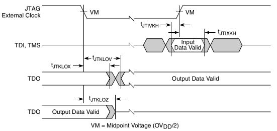
Figure 41. Test access port timing diagram
