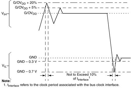
Figure 2. Overshoot/Undershoot voltage for GV<sub>DD</sub>/OV<sub>DD</sub>
