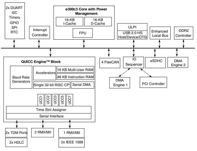
Figure 1. MPC8309 block diagram
