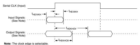
Figure 21. AC timing (external clock) diagram
