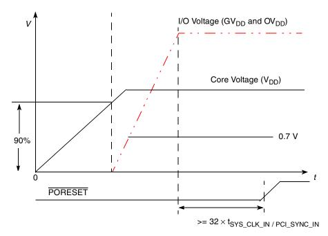
Figure 3. MPC8309 Power-Up sequencing example
