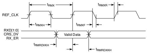
Figure 16. RMII receive AC timing diagram
