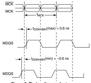
Figure 5. Timing diagram for  $t_{\text{DDKHMH}}$
