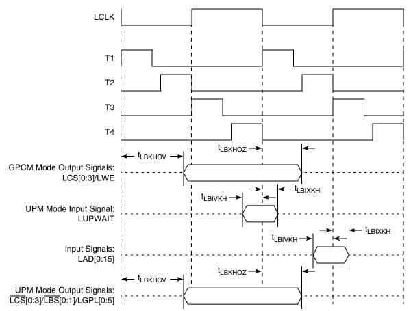
Figure 10. Enhanced local bus signals, GPCM/UPM Signals for LCRR[CLKDIV] = 4
