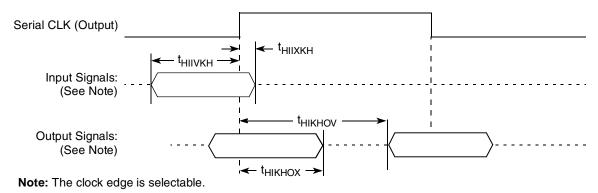
Figure 22. AC timing (internal clock) diagram
