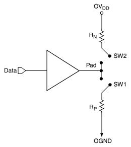
Figure 45. Driver impedance measurement
