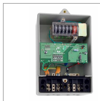
FIGURE 2-2: Photograph of Complete, Stand-Alone MCP3905A Energy Meter.
