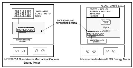
**FIGURE 2-1:** MCP3905A Stand-Alone Energy Meter and Microcontroller-Based Energy Meter Using MCP3905A AFE Design.
