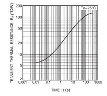
Fig.10 Transient thermal resistance
