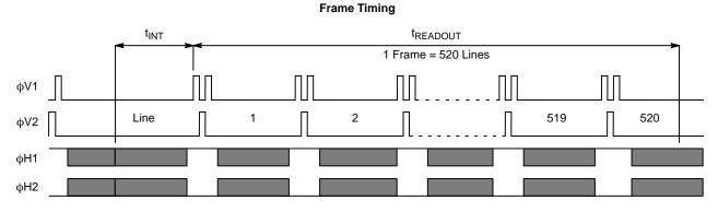
Figure 9. Frame Timing Diagram
