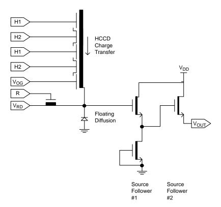
Figure 4. Output Schematic
