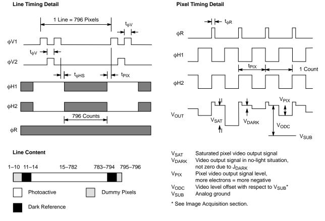
Figure 10. Line and Pixel Timing Diagrams
