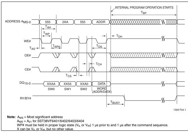
Figure 7: WE# Controlled Program Cycle Timing Diagram
