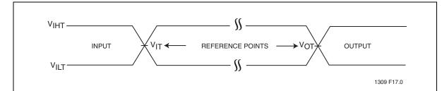
AC test inputs are driven at  $V_{IHT}$  (0.9  $V_{DD}$ ) for a logic "1" and  $V_{ILT}$  (0.1  $V_{DD}$ ) for a logic "0". Measurement reference points for inputs and outputs are  $V_{IT}$  (0.5  $V_{DD}$ ) and  $V_{OT}$  (0.5  $V_{DD}$ ). Input rise and fall times (10%  $\leftrightarrow$  90%) are <5 ns.
