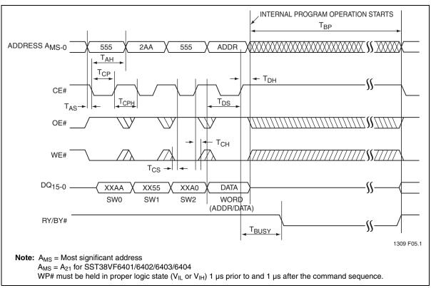
Figure 8: CE# Controlled Program Cycle Timing Diagram
