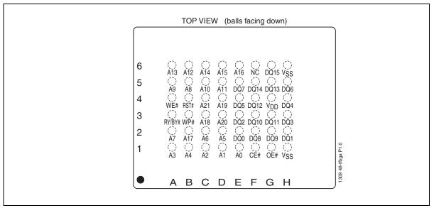
Figure 3: Pin assignments for 48-ball TFBGA
