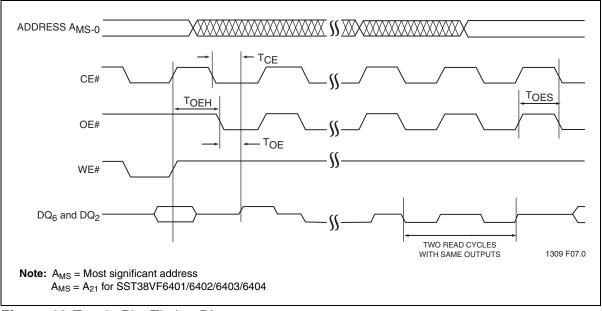
Figure 12: Toggle Bits Timing Diagram
