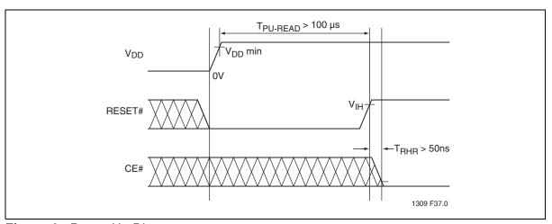
Figure 4: Power-Up Diagram
