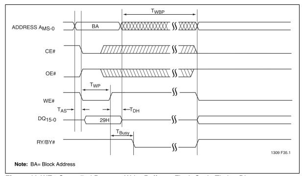
Figure 10:WE# Controlled Program-Write-Buffer-to-Flash Cycle Timing Diagram
