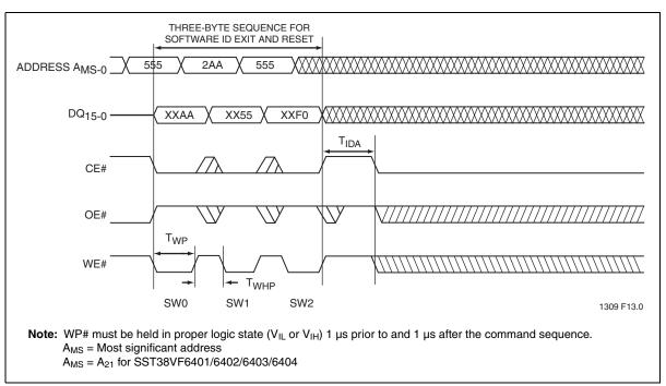
Figure 18: Software ID Exit/CFI Exit
