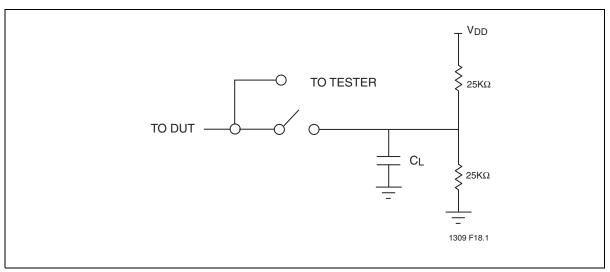
Figure 23:A Test Load Example
