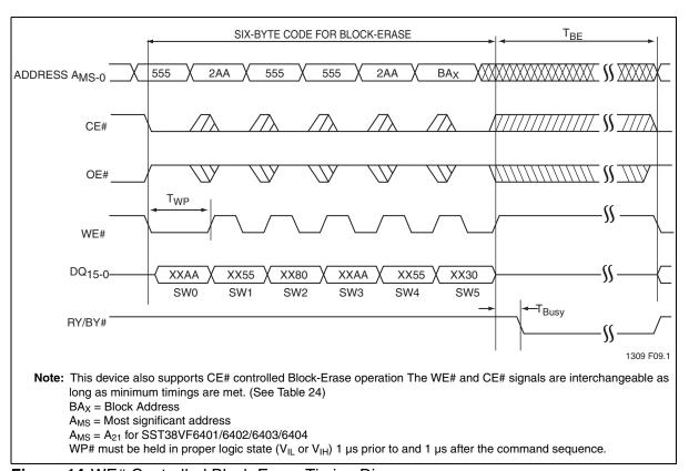
Figure 14:WE# Controlled Block-Erase Timing Diagram
