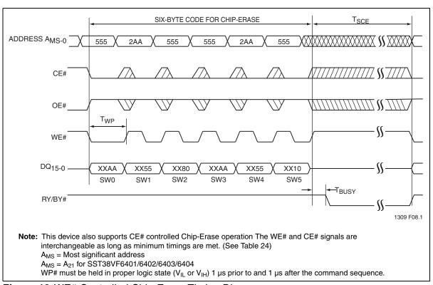
Figure 13:WE# Controlled Chip-Erase Timing Diagram
