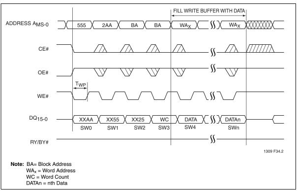
Figure 9: WE# Controlled Write-Buffer Cycle Timing Diagram
