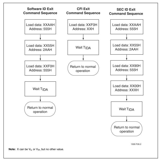
Figure 28: Software ID/CFI/SEC ID Exit Command Flowcharts
