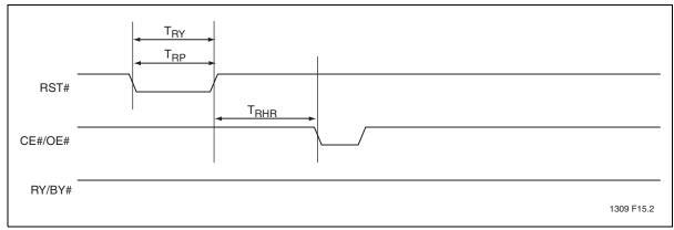
Figure 20:RST# Timing Diagram (When no internal operation is in progress)
