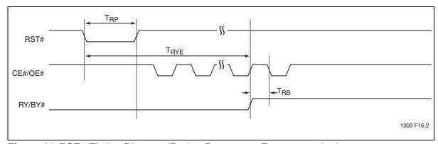
Figure 21:RST# Timing Diagram (During Program or Erase operation)
