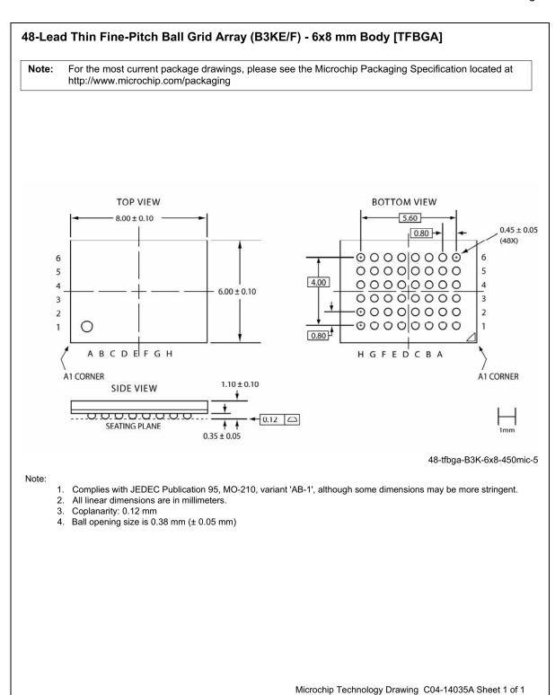
**Figure 37:**48-ball Thin-profile, Fine-pitch Ball Grid Array (TFBGA) 6mm x 8mm Package Code: B3KE
