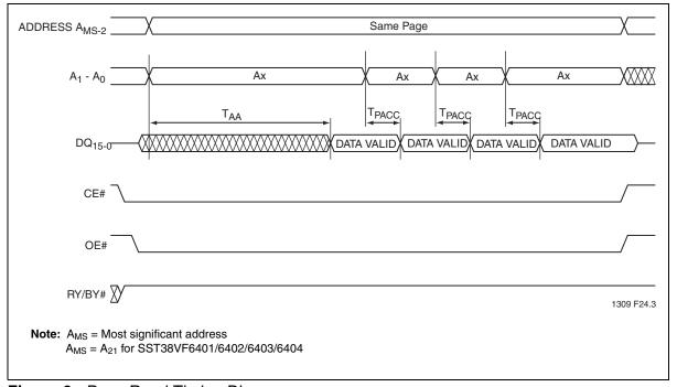
Figure 6: Page Read Timing Diagram
