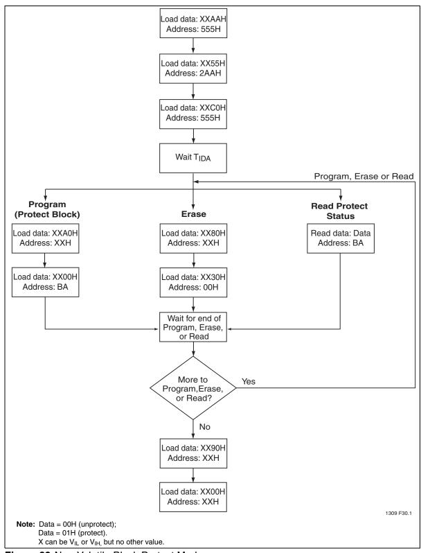
Figure 32: Non-Volatile Block Protect Mode
