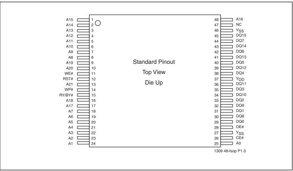
Figure 2: Pin Assignments for 48-lead TSOP
