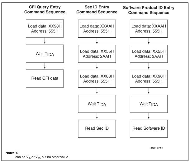
Figure 27:CFI/SEC ID/Software ID Entry Command Flowcharts
