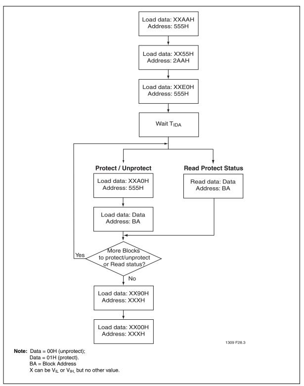
Figure 31: Volatile Block Protection
