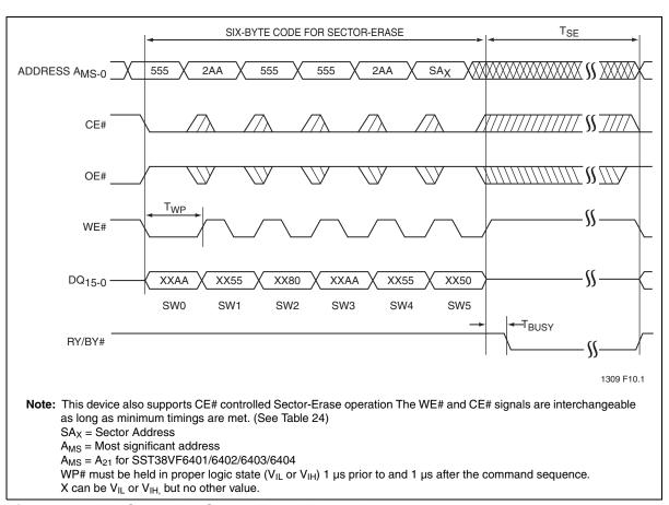
Figure 15:WE# Controlled Sector-Erase Timing Diagram
