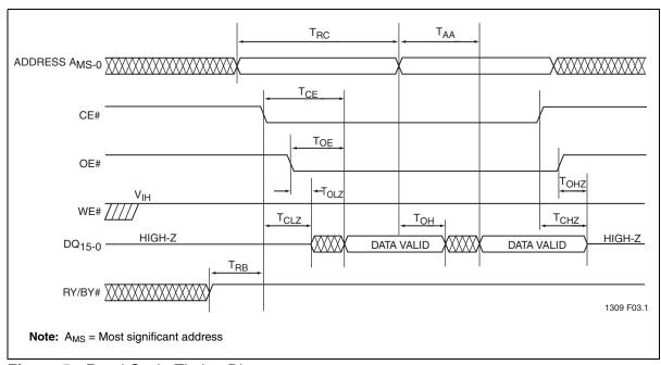
Figure 5: Read Cycle Timing Diagram
