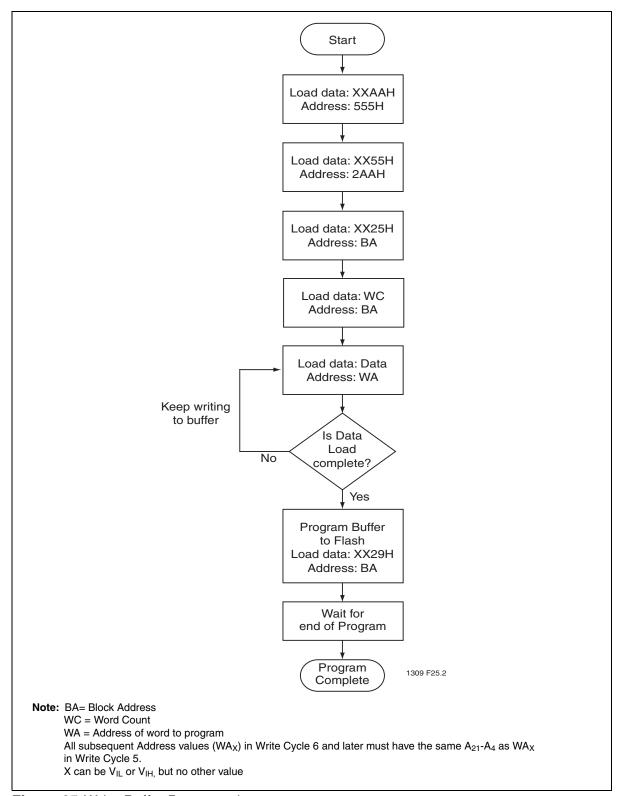
Figure 25: Write-Buffer Programming
