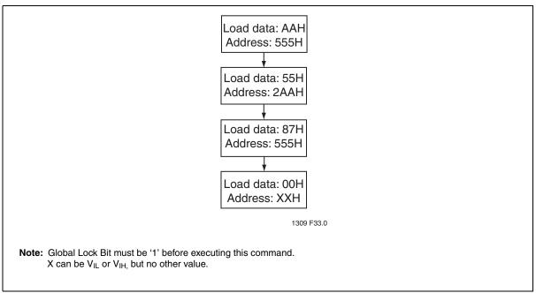
Figure 35: Irreversible Block Lock in Main Array
