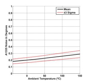
Figure 24: Noise Performance over Temperature (1 Sigma, 300 G)
