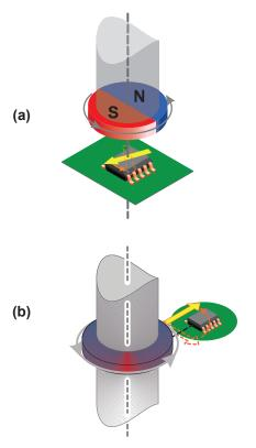
Figure 12: Typical On-Axis (a) and Off-Axis (b) Orientation
