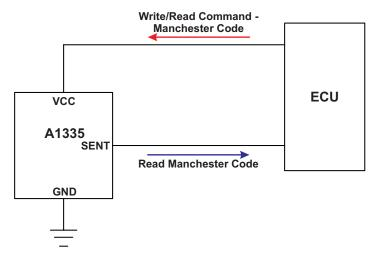
Figure 3: Top-Level Programming Interface
