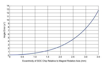
Figure 11: Simulated Error versus Eccentricity for a 10 mm × 4 mm Neodymium magnet at a 2.7 mm air gap.
