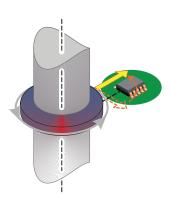
Industry-leading linearization enables off-axis (side-shaft) operation
