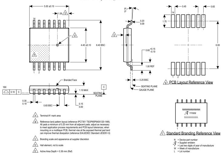
Figure 27: Package LE, 14-Pin TSSOP (Single Die Version)
