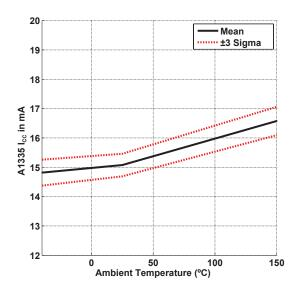
Figure 26:  $I_{CC}$  over Temperature  $(V_{CC} = 5.5 \text{ V})$
