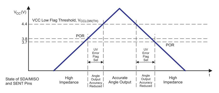
Figure 2: Relationship of V<sub>CC</sub> and Output
