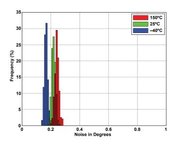
Figure 23: Noise Distribution over Temperature  $(V_{CC} = 5.5 \text{ V})$
