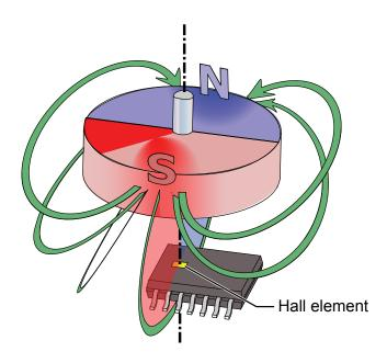
Figure 15: Centering the axis of magnet rotation on the Hall element provides the strongest signal in all degrees of rotation.
