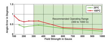
Figure 9: Typical Maximum Angle Error
