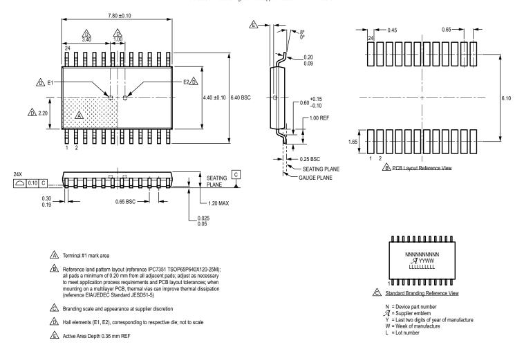
Figure 28: Package LE, 24-Pin TSSOP (Dual Die Version)
