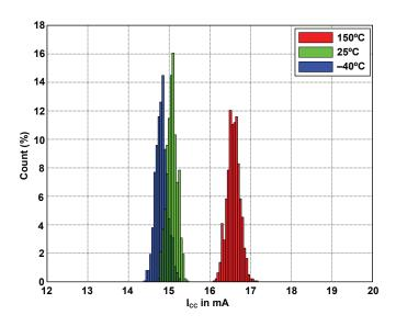
Figure 25:  $I_{CC}$  Distribution over Temperature  $(V_{CC} = 5.5 \text{ V})$
