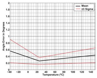
Figure 21: Peak Angle Error over Temperature (300 G)
