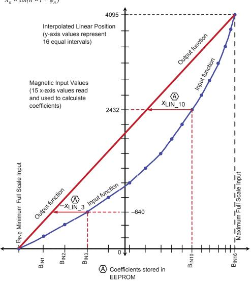
Figure 19: Sample of Linearization Function Transfer Characteristic
