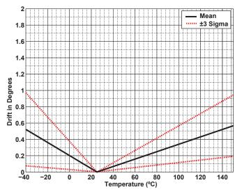
Figure 22: Maximum Absolute Drift from 25°C Reading (300 G)
