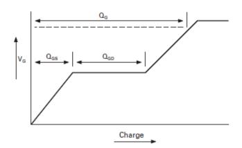
Basic gate charge waveform
