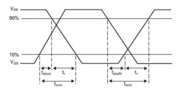
Switching time waveforms
