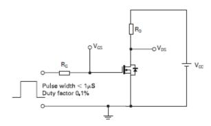
Switching time test circuit
