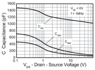
Capacitance v Drain-Source Voltage
