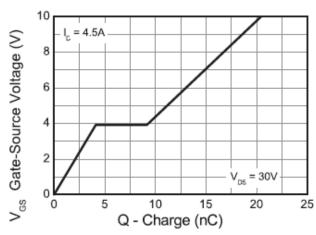
Gate-Source Voltage v Gate Charge
