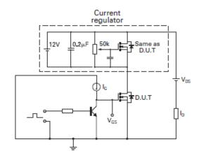
Gate charge test circuit
