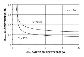
Figure 4. On-Resistance Variation with Gate-to-Source Voltage.
