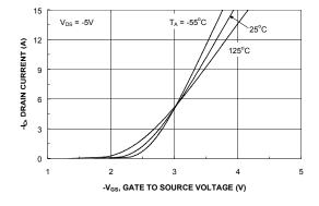
Figure 5. Transfer Characteristics.
