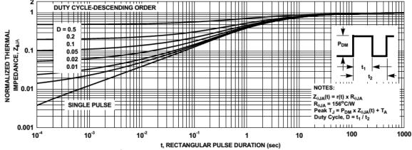
Thermal characterization performed using the conditions described in Note 1b. Transient themal response will change depending on the circuit board design.
