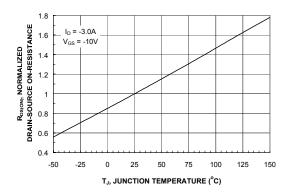
Figure 3. On-Resistance Variation with Temperature.
