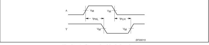
Waveform 1. Propagation delay for inverting outputs
