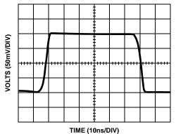
FIGURE 19. SMALL SIGNAL RISE AND FALL TIME
