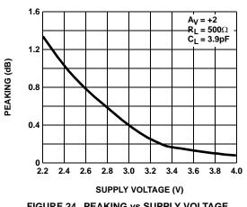
FIGURE 24. PEAKING vs SUPPLY VOLTAGE
