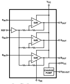
$V_{OUT} = 2V_{IN} - V_{REFERENCE}$
