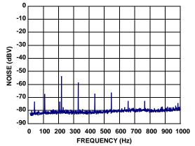
FIGURE 21. NOISE FLOOR WITH CHARGE PUMP HARMONICS
