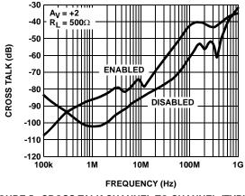
FIGURE 5. CROSS TALK CHANNEL TO CHANNEL (TYPICAL)
