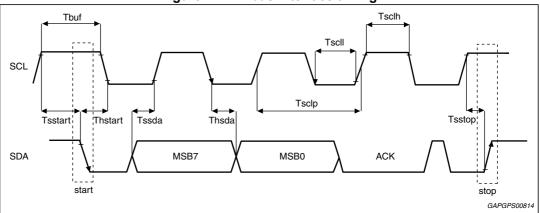
Figure 72. I<sup>2</sup>C bus interface timing
