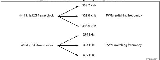
Figure 60. PWM switching frequency selection
