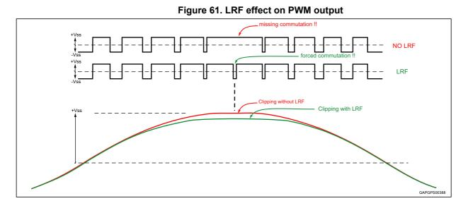
Please note that, by limiting the PWM duty cycle, a limitation of the output power occurs: the output power in case of usage of LRF function decreases about 10 % @ 1 % THD.
