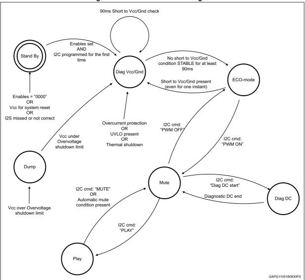
Figure 38. Finite state machine diagram
