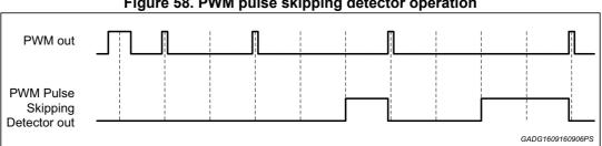
Figure 58. PWM pulse skipping detector operation
