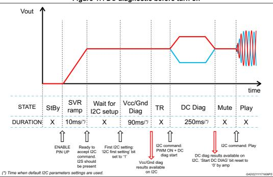
Figure 47. DC diagnostic before turn on
