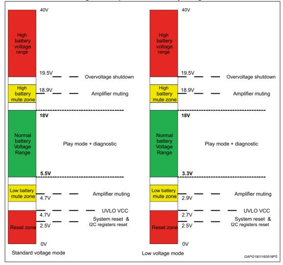
Figure 39. Operation vs. battery charge
