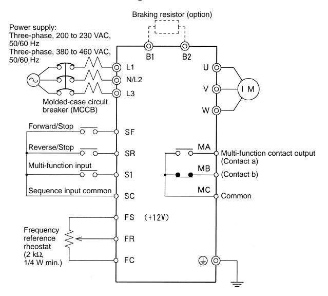
**Note 1.** If a 3G3EV-AB□□□ is used in single-phase input mode, single-phase 200 to 240 VAC power with a frequency of 50/60 Hz must be input between terminals R and S.
