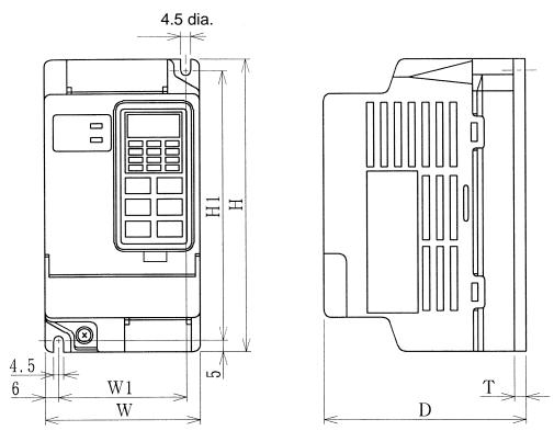
**Note 1.** For the 3G3EV-A2001(-□), 3G3EV-A2002(-□), and 3G3EV-AB001(-□), a U-shaped notch (4.5 mm wide) is provided instead of the upper mounting hole (4.5 mm in diameter).
