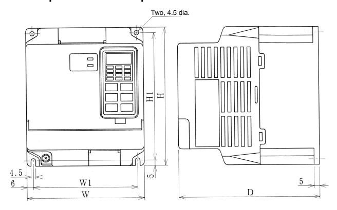
Note Install the Inverter with four M4 bolts.
