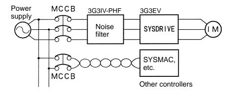
**Note** Use a special-purpose noise filter for Inverters.
