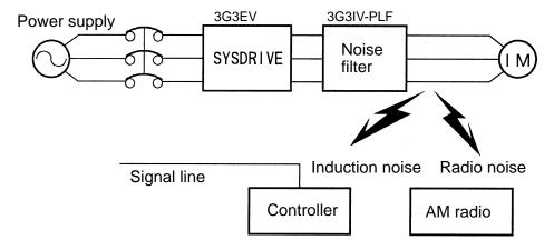
Induction Noise: Electromagnetic induction generates noise on the signal line, causing
