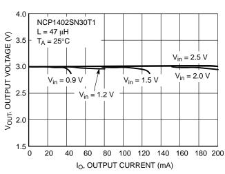
Figure 4. NCP1402SN30T1 Output Voltage vs.
