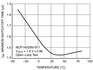
Figure 18. NCP1402SN19T1 Minimum Switch Off Time vs. Temperature
