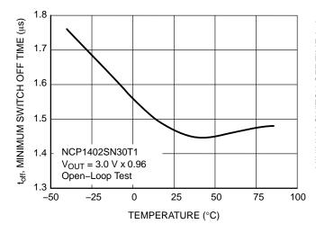
Figure 19. NCP1402SN30T1 Minimum Switch Off Time vs. Temperature
