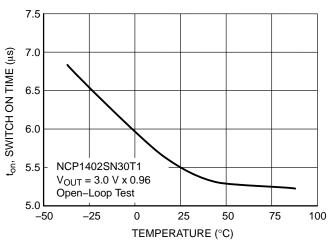
Figure 16. NCP1402SN30T1 Switch On Time vs. Temperature
