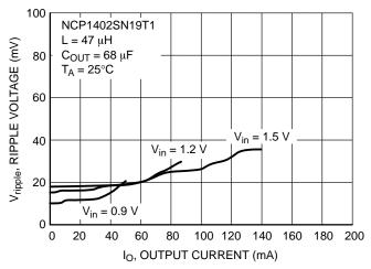
Figure 51. NCP1402SN19T1 Ripple Voltage vs.
