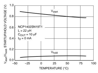
V<sub>start</sub>/V<sub>hold</sub>, STARTUP/HOLD VOLTAGE (V) V<sub>start</sub> 0.8 NCP1402SN30T1 0.6  $L = 22 \mu H$  $C_{OUT} = 10 \mu F$  $I_O = 0 \text{ mA}$ 0.4 0.2  $V_{hold}$ -25 0 25 50 75 100 -50 TEMPERATURE (°C)
