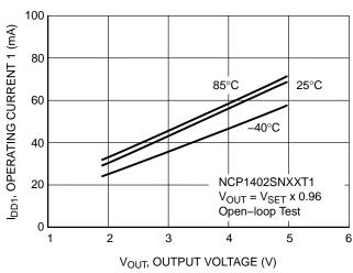
Figure 54. NCP1402SNXXT1 Operating Current 1 vs. Output Voltage
