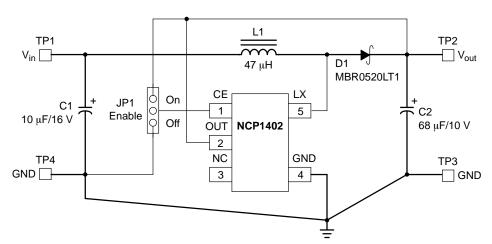
Figure 62. NCP1402 Evaluation Board Schematic Diagram
