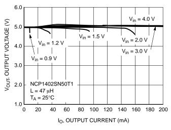
Figure 5. NCP1402SN50T1 Output Voltage vs. Output Current
