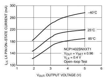
Figure 55. NCP1402SNXXT1 Pin On-state Current vs. Output Voltage
