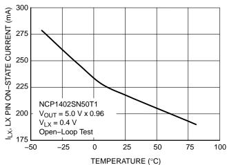
Figure 25. NCP1402SN30T1 LX Pin On–State Current vs. Temperature
