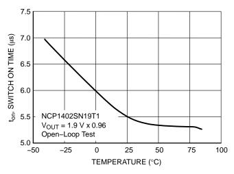
Figure 15. NCP1402SN19T1 Switch On Time vs. Temperature
