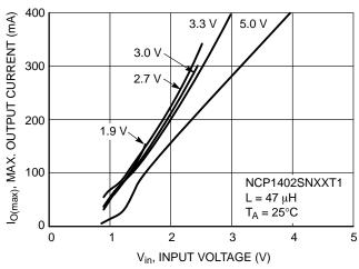
Figure 58. NCP1402SNXXT1 Maximum Output Current vs. Input Voltage
