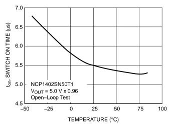
Figure 17. NCP1402SN50T1 Switch On Time vs. Temperature
