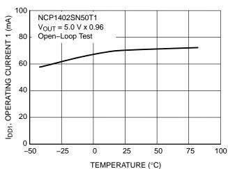
Figure 13. NCP1402SN30T1 Operating Current 1 vs. Temperature
