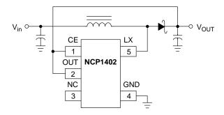
Figure 1. Typical Step-Up Converter Application
