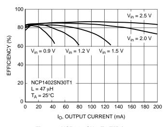
Figure 7. NCP1402SN30T1 Efficiency vs.
