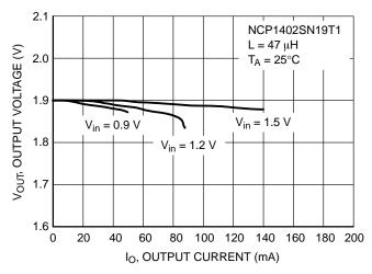
Figure 3. NCP1402SN19T1 Output Voltage vs.
