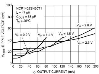
Figure 52. NCP1402SN30T1 Ripple Voltage vs.
