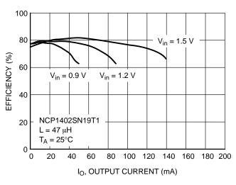
Figure 6. NCP1402SN19T1 Efficiency vs.
