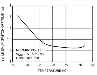
Figure 20. NCP1402SN50T1 Minimum Switch Off Time vs. Temperature
