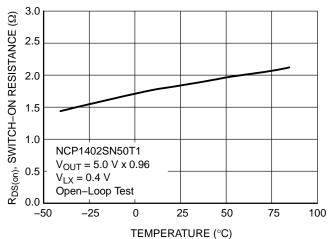
Figure 31. NCP1402SN30T1 Switch-on Resistance vs. Temperature
