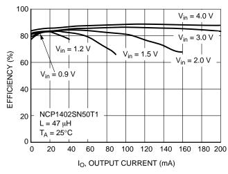
Figure 8. NCP1402SN50T1 Efficiency vs.
