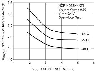
Figure 56. NCP1402SNXXT1 Switch-On Resistance vs. Output Voltage
