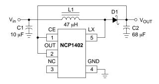
Figure 59. Typical Application Circuit
