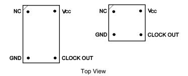
Figure 2-4. Mapping of Oscillator to Socket
