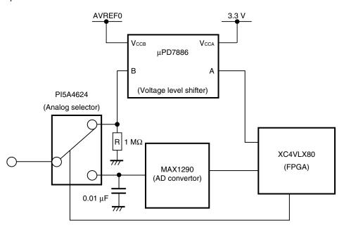
Figure A-1. Equivalent Circuit of Target Interface (2/6)
