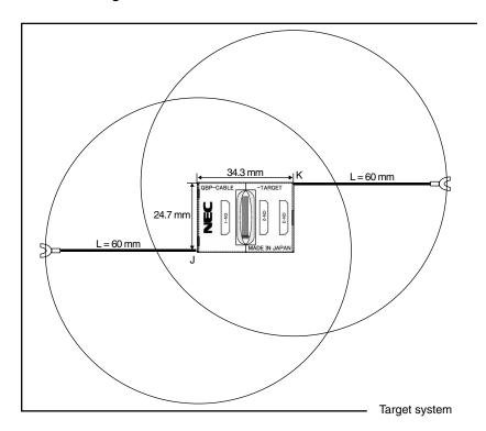
Figure 2-7. Where GND Wire Can Be Connected
