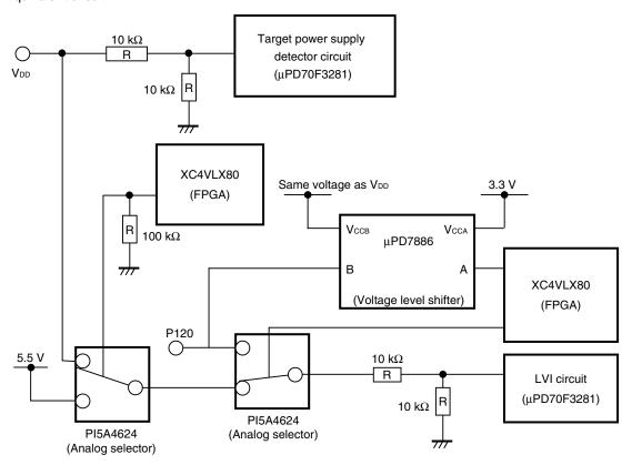
Figure A-1. Equivalent Circuit of Target Interface (3/6)
