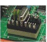
Figure 2-3. Oscillator Shape
