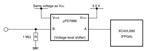
Figure A-1. Equivalent Circuit of Target Interface (4/6)
