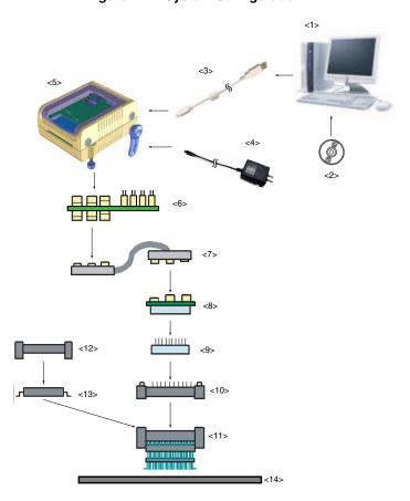
Figure 1-1. System Configuration
