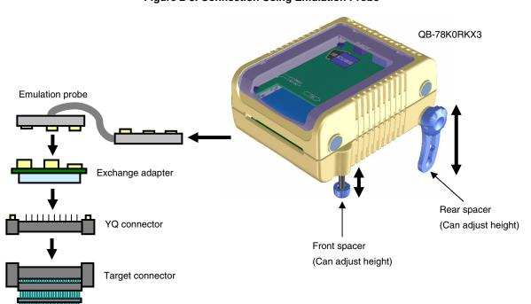
Figure 2-8. Connection Using Emulation Probe
