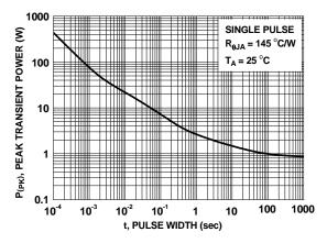
Figure 10. Single Pulse Maximum Power Dissipation
