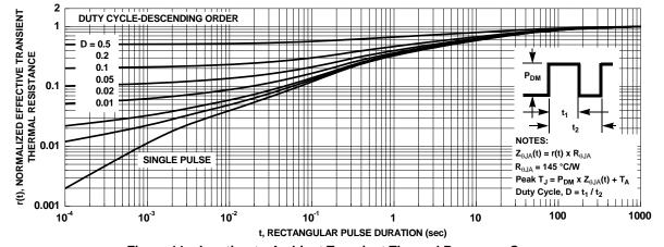
Figure 11. Junction-to-Ambient Transient Thermal Response Curve
