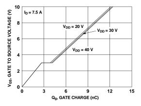
Figure 7. Gate Charge Characteristics
