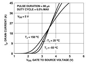
Figure 5. Transfer Characteristics
