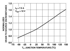
Figure 3. Normalized On-Resistance vs Junction Temperature
