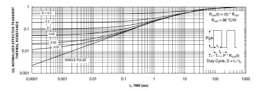
Figure 11. Transient Thermal Response Curve.
