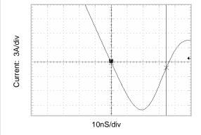
Figure 12. FDD6680AS SyncFET body diode reverse recovery characteris
