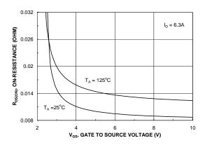
Figure 4. On-Resistance Variation with Gate-to-Source Voltage.
