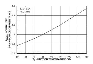
Figure 3. On-Resistance Variation with Temperature.
