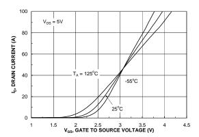
Figure 5. Transfer Characteristics.
