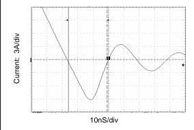
Figure 13. Non-SyncFET (FDD6680) body diode reverse recovery characteristic.
