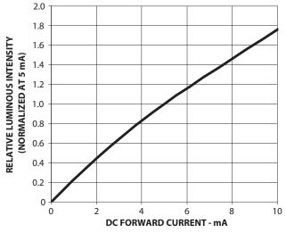
Figure 3. Luminous intensity vs. forward current
