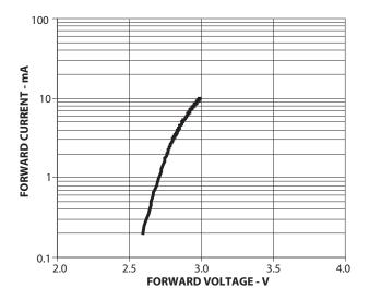
Figure 2. Forward voltage vs. forward current
