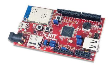
Building on the previous successes with the chipKIT WF32, the Wi-FIRE uses the same 43 available I/O pins, 12 analog inputs, 3.3 operating voltage, 4 user LEDs, potentiometer, buttons, uses MRF24 on-board wireless module, microSD Card, dedicated SPI Signals and high efficiency switching 3.3V switching power supply for low-power operation. Where the boards differ is in what the PIC32MZ processor can deliver.
